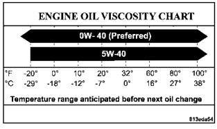
The engine oil filler cap also shows the recommended engine oil viscosity for your engine. For information on engine oil filler cap location, refer to the "Engine Compartment" illustration in this section.
